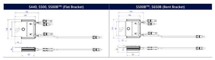
(10) S500B has either a flat bracket or a bent bracket. S500B-1GM4MRM has a flat bracket, and S500B-1GM4MBM has a bent bracket.
