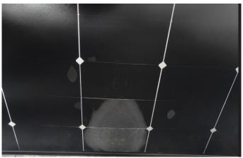
Supplementary information: The backpanel has broken, but nothing has been blown off or fallen off the test deck in the form of flaming or growing brands.
