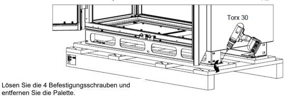
Loosen the 4 fastening screws and remove the pallet.
