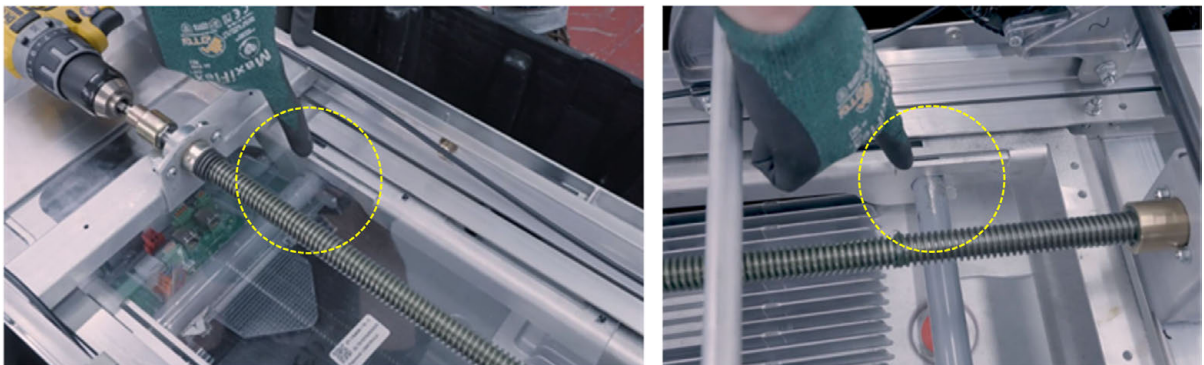
Figure 4. Lift Handles Securely Locked to the Locking Plate on Top and Bottom
